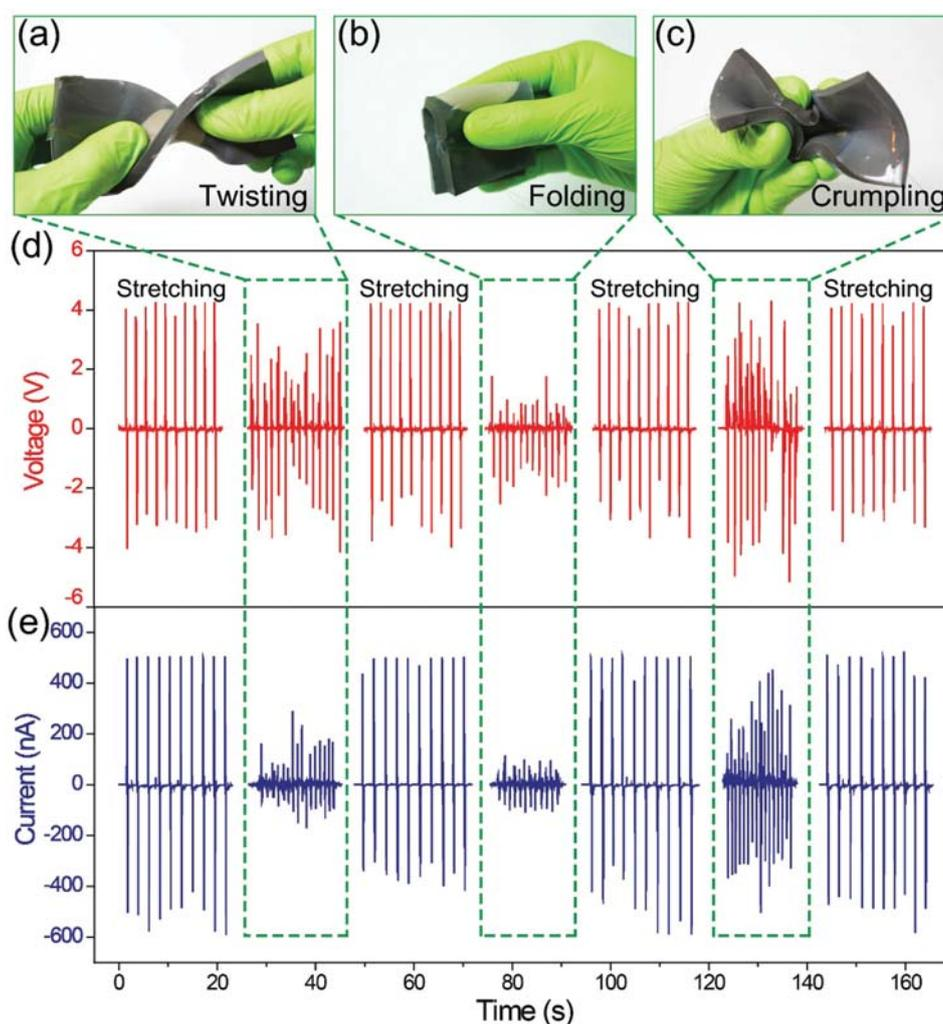
**Figure 4.** a–c) Photographs of the SEG when subjected to various deformations, such as twisting, folding, and crumpling, which can be converted into corresponding electricity: d) voltage and e) current. These energy-harvesting properties are also shown in Video S1 in the Supporting Information.
