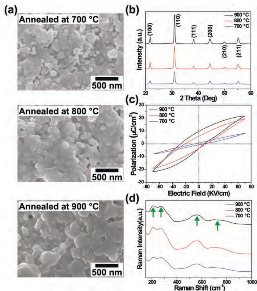
**Figure 2.** a) Top-view SEM images of AD PZT thick films deposited on sapphire substrates and annealed at temperatures of 700, 800, and 900 °C. b) XRD patterns of AD PZT thick films annealed at three different temperatures. c) Polarization–electric ( $P$ - $E$ ) hysteresis loops of the flexible ferroelectric PZT films as a function of annealing temperature at room temperature. d) Raman spectra of the high-temperature-annealed AD PZT films transferred onto PET substrates.
