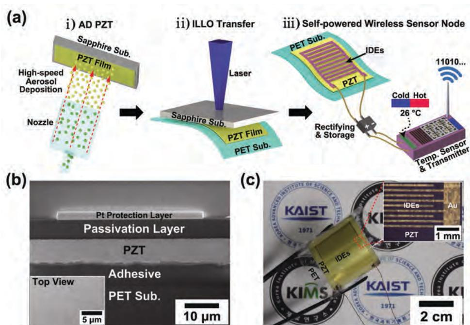
**Figure 1.** a) Schematic illustration of the device-fabrication process and self-powered WSN using a flexible AD PZT energy harvester enabled by ILLO. b) A cross-sectional SEM image of the AD PZT thick film on a PET substrate. The inset shows a top-view SEM image of the flexible PZT thick film. c) An optical image of the flexible PZT harvester bent by tweezers. The inset shows a top-view OM image of metal IDEs on the PZT.
