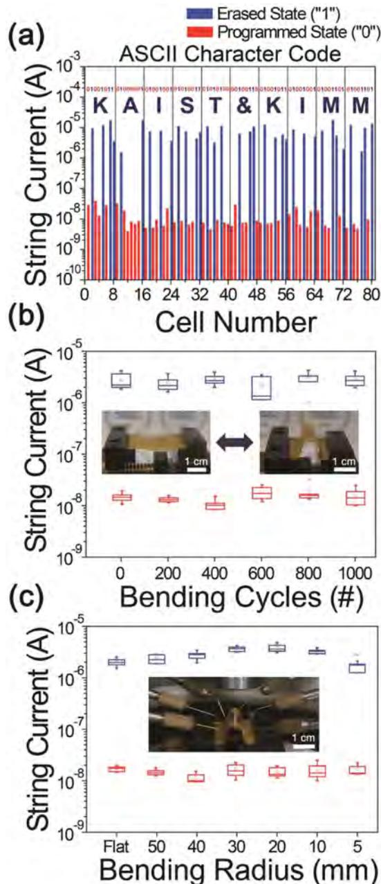
**Figure 5.** a) The NAND flash string current histogram showing the words “KAIST&KIMM” with standard ASCII character codes within the 80 bit flexible NAND flash memory. b) Bending fatigue test results of the flexible NAND flash memory during 1000 bending cycles. c) The string current of the programmed and erased states as a function of bending radius. (Erased state “1” and programmed state “0” are denoted by blue and red, respectively, for all of (a), (b), and (c).)
