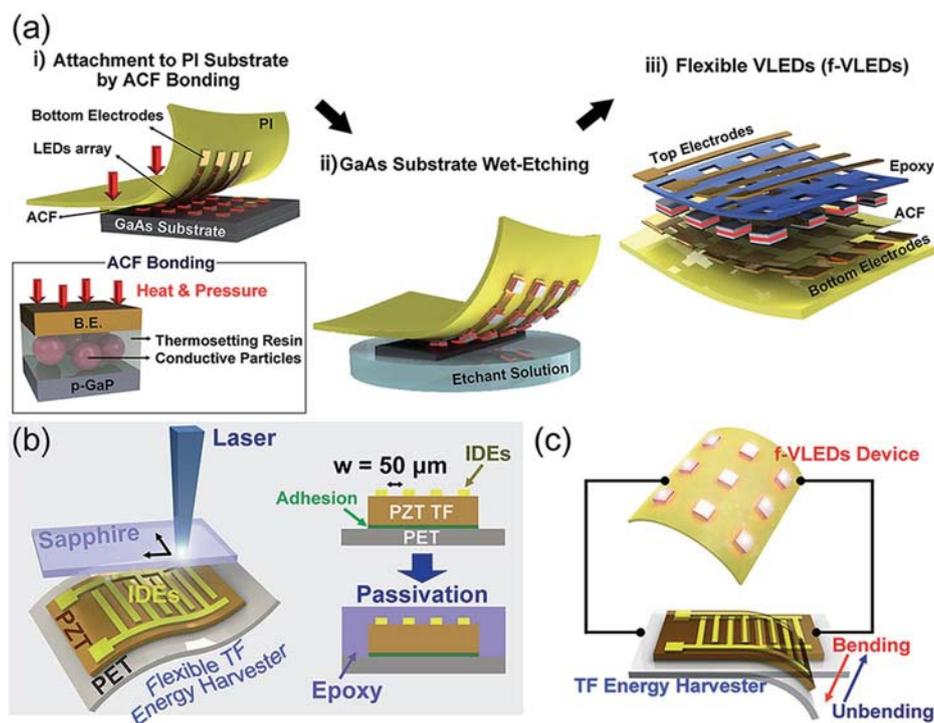
Fig. 1 Schemes for a self-powered flexible light-emitting system. Illustrations showing the fabrication steps of: (a) red emitting f-VLEDs with MQW layers; and (b) a flexible thin-film (TF) energy harvester. (c) Schematics of the final self-powered flexible light-emitting system.
