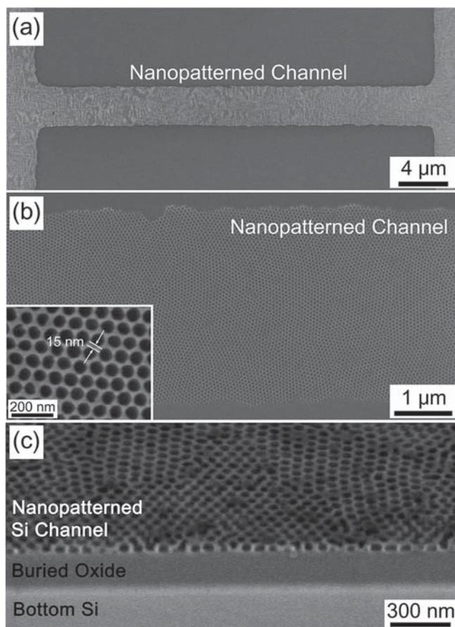
**Figure 2.** a) SEM image of a nanopatterned Si channel. Moiré fringes over the entire channel region demonstrate the uniformity of the nanopatterned Si structure. b) Magnified SEM image of the nanopatterned Si channel. c) Cross-sectional SEM image of the hexagonal nanohole morphology of the top Si layer ( $\approx 25$  nm thickness).
