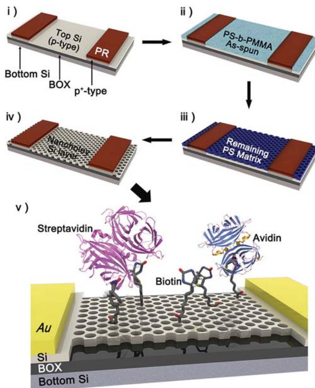
**Figure 1.** Schematic process for a nanopatterned electrical biosensor, including i) boron doping, ii) BCP spin-casting and self-assembly, iii) PMMA domain removal, and iv) pattern transfer to the top Si layer. v) An FET-based biosensor is functionalized with biotin molecules for detecting streptavidin or avidin protein (BOX = buried oxide).
