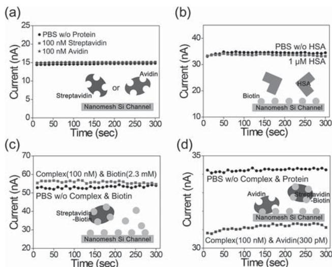
**Figure 6.** a) Current levels of the nanomesh channel without biotinylation. b) Current characteristics of the biotinylated nanomesh device with the nonspecific protein, HSA. c) Current levels of the nanopatterned and biotinylated channel in the presence of excess biotin molecules and preblocked streptavidin–biotin complex. d) Current change of the biotinylated nanomesh Si channel upon mixing the solution with 300 pM avidin and preblocked streptavidin–biotin complex.
