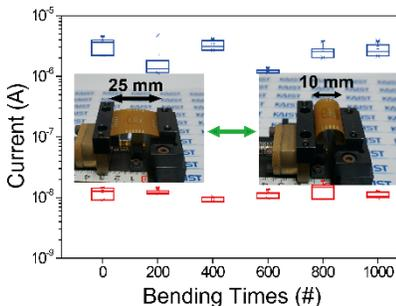
**Fig. 21.** Bending fatigue test results of the flexible NAND flash memory during 1000 bending cycles. The inset shows photographs of the bending and unbending states.
