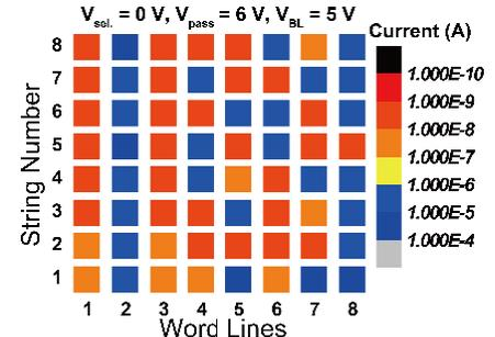
**Fig. 19.** Color map of the string current distribution based on the memory state of the 64 cells in the  $8 \times 8$  array. To verify the string current difference between erased and programmed states, the read operation was carried out with  $V_{sel} = 0$  V,  $V_{pass} = 6$  V, and  $V_{BL} = 5$  V.
