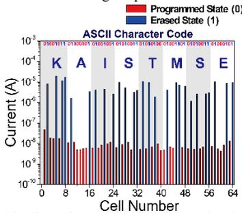
**Fig. 20.** The string current histogram showing the words "KAIST MSE" with standard ASCII characters within the 64 bit flexible NAND flash memory.
