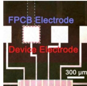
**Fig. 4.** Optical microscope image of the electrode area where the FPCB electrode and the device electrode are interconnected.
