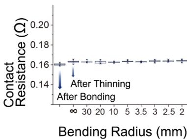
**Fig. 8.** Measured contact resistance with varying bending radius. No significant resistance increase was observed until it reached a 2 mm bending radius.
