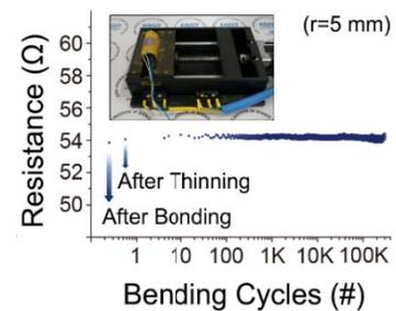
**Fig. 10.** Measured 144-series daisy-chain resistance with repetitive bending. No significant resistance increase was observed during  $3 \times 10^5$  iterations (5 mm radius) of bending.
