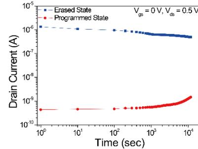
**Fig. 16.** Retention characteristics of the flexible flash memory.
