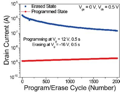
**Fig. 15.** Endurance test of the flexible flash memory measured during more than 2000 cycles.
