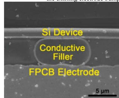
**Fig. 7.** Cross-sectional scanning electron microscopy image of the ultrathin Si device interconnected to the flexible substrate (FPCB) by a conductive filler ball.
