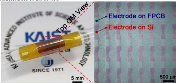
**Fig. 6.** Optical image of the ACF-packaged ultrathin Si-based flexible chip used for electrical measurement (left) and a magnified top-view image of the 144-series daisy-chain (right). (Electrode area = 1802  $\mu\text{m}^2$ .)
