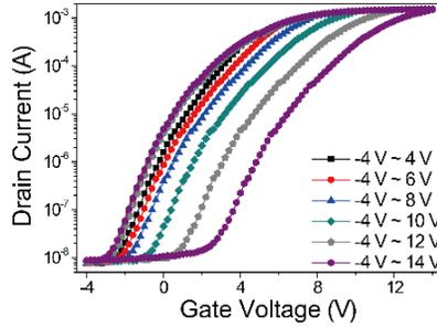
**Fig. 12.** The charge trap memory characteristics of the flexible flash memory. Voltage pulses of -16 V/0.5 s were applied to the gate for erasing, in order to obtain double transfer curves with increasing maximum gate voltages.
