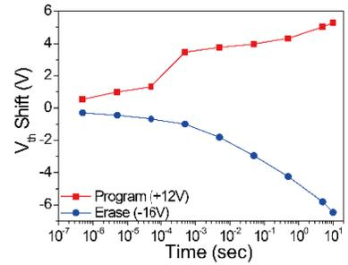
**Fig. 13.** The  $V_{th}$  shift plots of the flexible flash memory as a function of the voltage pulse widths. The  $V_{th}$  shifts were increased with increasing erase/program operation times.
