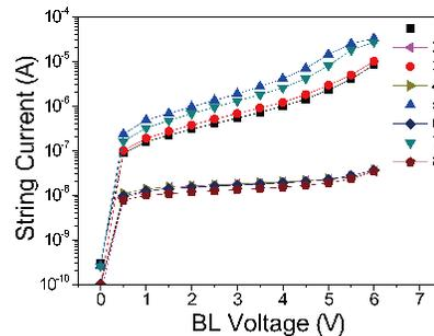
**Fig. 18.** The string current of the flexible NAND flash string according to the address number of memory cells. There is a distinct difference in the string current between the programmed and erased cells.
