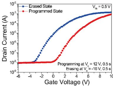
**Fig. 14.** The transfer curves of the programmed and erased states were measured at  $V_d = 0.5$  V. This memory device exhibited a high on/off at  $V_g = 0$  V (reading voltage for a selected memory cell in the NAND logic gate).
