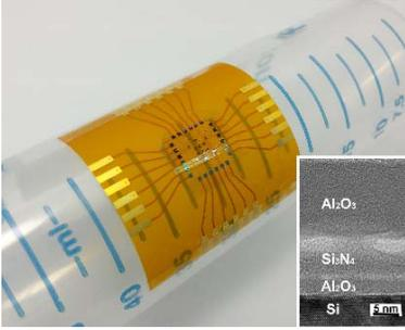
**Fig. 11.** A photograph of the ACF-packaged Si-based flexible flash memories on flexible substrate. The inset shows a cross-sectional TEM image of the  $\text{Al}_2\text{O}_3/\text{Si}_3\text{N}_4/\text{Al}_2\text{O}_3$  multilayer thin films deposited on the silicon to fabricate the flash memory.
