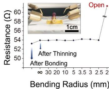
**Fig. 9.** Measured 144-series daisy-chain resistance with varying bending radius. (The slightly high initial resistance is caused by the resistance of the thin electrode fabricated on the Si chip rather than the interconnection resistance.) No significant resistance increase was observed until it was bent to a 2.5 mm bending radius.
