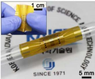
**Fig. 2.** Photograph of the fabricated ACF-packaged ultrathin Si-based flexible NAND flash memory wrapped on a glass rod (3.5 mm radius). The inset shows the highly flexible characteristics of the device.
