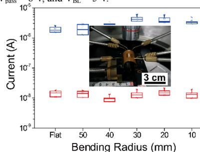
**Fig. 22.** The string current of the programmed and erased states as a function of bending radius. The inset is a photograph of the string current measurement under a flexed condition.
