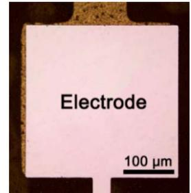
**Fig. 5.** Optical microscope image of the electrode area. No cracks or wrinkles were observed in spite of the height difference caused by the existing electrode bump.
