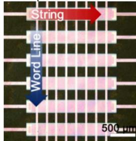
**Fig. 3.** Optical microscope image of the Si-based flexible NAND flash active area, with no cracks or wrinkles.
