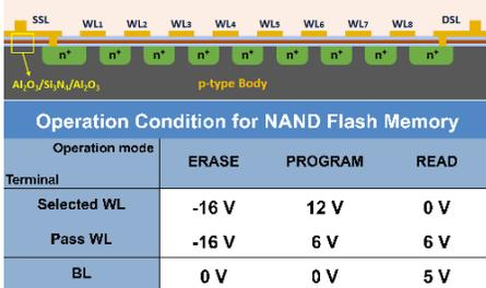
**Fig. 17.** Schematic illustration of a cross-sectional view of a Si-based flexible NAND flash memory. The Si-based transistors with  $\text{Al}_2\text{O}_3/\text{Si}_3\text{N}_4/\text{Al}_2\text{O}_3$  stacks have been assembled into a series string of 8 memory MOSFETs. Operation conditions for the NAND flash cell string are presented below.
